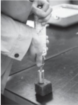
Foto 7. Needle Penetrating Test.
