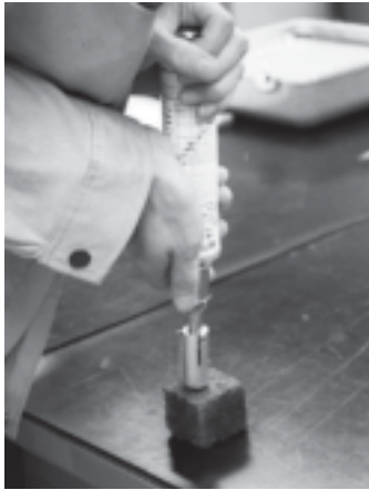
Foto 7. Needle Penetrating Test.
